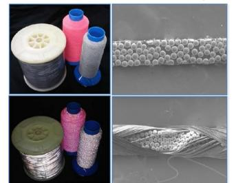
HJLite Reflective Yarns / Threads are composed of retroreflective lenses (glass beads) bonded to film and slit to very narrow widths. They may be woven directly into ribbon, trim, piping, laces, and fabrics to achieve a variety of reflective patterns.
